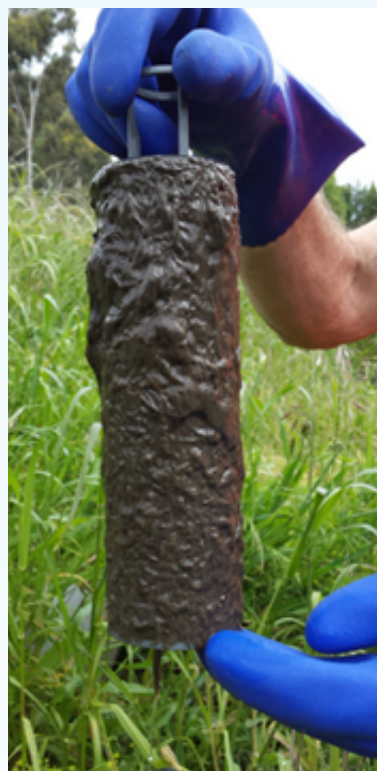
Excessive filter clogging due to poor treatment plant performance
