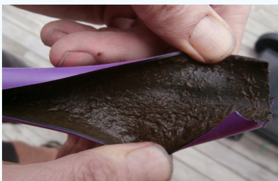
Drip lines must be regularly flushed to prevent biofilm build-up and blockage
