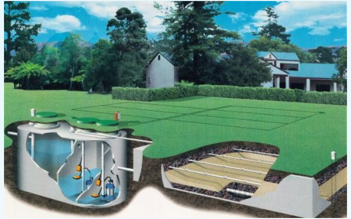
Modern septic tank, sand filter and drip irrigation field
